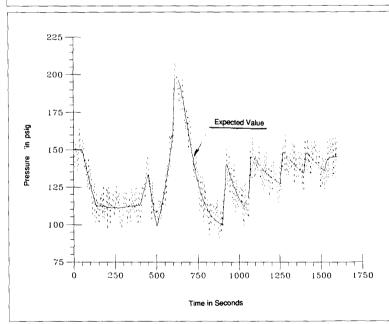
Fig. 7. Dearator pressure transients using the reconfigurable scheme (with noisy measurements).
