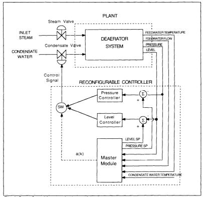
Fig. 1. Reconfigurable control scheme of the deaerator.
