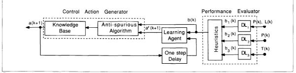
Fig. 2. Internal structure of the master module.
