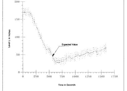
Fig. 8. Deaerator level transients using the reconfigurable scheme (with noisy measurements).
