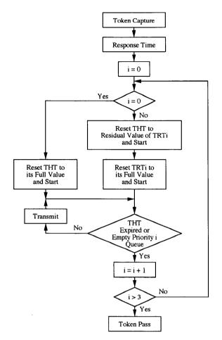
Fig. 6. Priority mechanism of LTPB protocol.
