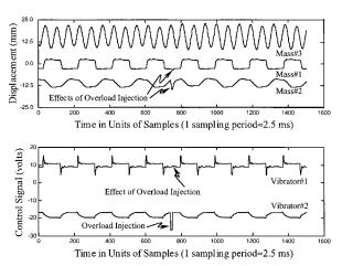
Fig. 3 Impact of overload injection on system performance
