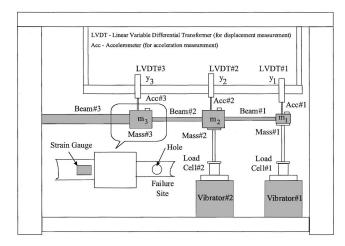
Fig. 1 Schematic diagram of the test apparatus
