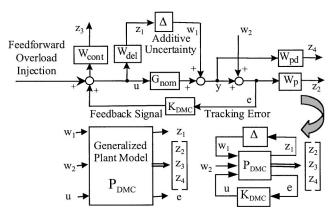
Fig. 2 Linear robust control system
