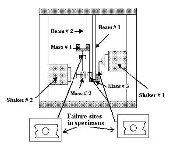
Fig. 1. Schematic diagram for the test apparatus.
