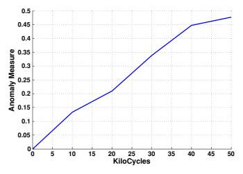
Figure 7. Fatigue damage evolution during crack initiation.
