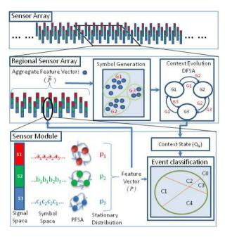
Fig. 1: Schematic representation of the proposed framework
