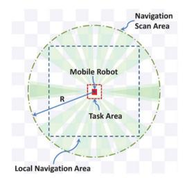
Figure 2. Autonomous vehicle and its sensing and computation areas.
