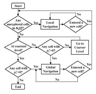
Figure 4. Flowchart of a multi-resolution navigation algorithm.
