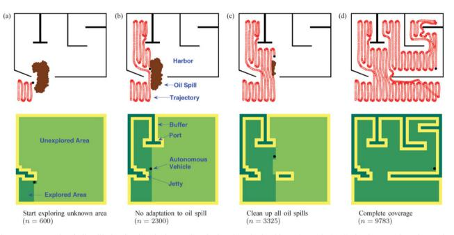
Figure 7. Example of oil spill cleaning in a harbour using the benchmark algorithm (Jin et al., 2012) that has no adaptation to the oil spill. (a) Start exploring unknown area (n = 600). (b) No adaptation to oil spill (n = 2300). (c) Clean-up all oil spills (n = 3325). (d) Complete coverage (n = 9783).
