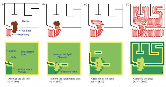
Figure 6. Example of oil spill cleaning in a harbour using the proposed multi-resolution navigation algorithm. (a) Discover the oil spill (n = 600). (b) Clean-up all oil spills (n = 2830). (c) Complete coverage (n = 10865). (d) Complete coverage (n = 10865).
