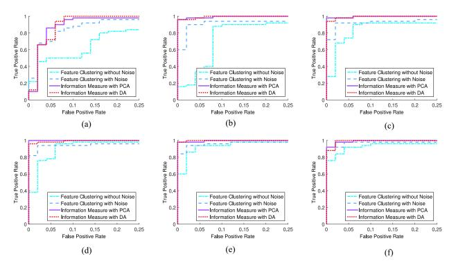
Fig. 7. ROC curves for target detection under different choices of the alphabet size. (a)  $|\mathcal{A}| = 3$ . (b)  $|\mathcal{A}| = 4$ . (c)  $|\mathcal{A}| = 5$ . (d)  $|\mathcal{A}| = 6$ . (e)  $|\mathcal{A}| = 7$ . (f)  $|\mathcal{A}| = 8$ .
