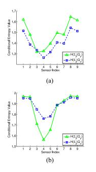
Fig. 5. Average conditional entropies for (a) target absent and (b) target present.
