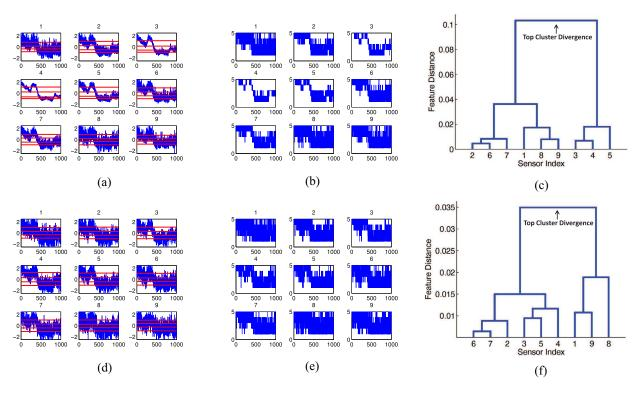
Fig. 4. Feature clustering with alphabet size  $|\mathcal{A}| = 5$  and cosine distance measurement used as the distance among PFSA features. Plates (a)–(c), respectively, show partitioning, symbolization, and feature clustering before noise injection. Plates (d)–(f), respectively, show the same after noise injection.
