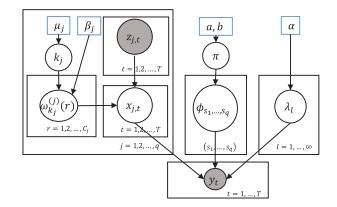
Fig. 1. Graphical representation of the Bayes network. The quantity enclosed by a rectangle represents a deterministic hyperparameter. The quantities enclosed by transparent circles denote unobserved random variables, while those enclosed by shaded circles denote observed random variables.
