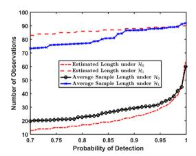
**Fig. 10.** Average sample length and estimated length for different values of  $p_d$  (max. 0.999) and constant  $p_{fa} = 0.01$ .
