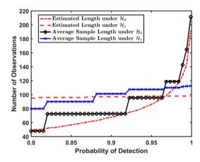
**Fig. 4.** Average sample length and estimated length for different values of desired probability of detection ( $p_d$ ) and constant probability of false alarm ( $p_{fa}$ ) = 0.001.
