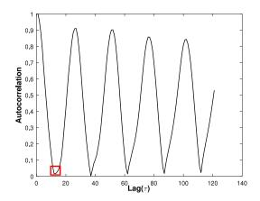
Fig. 8. Auto-correlation function of time-series data in the unstable phase of combustion. The time-series data is down-sampled by the lag marked in the red square. It is noted that the individual time-series have their own down-sampling lags.
