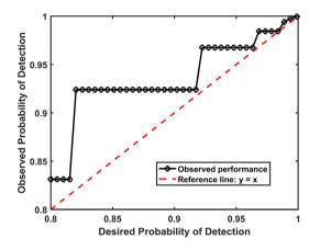
**Fig. 6.** Observed probability of detection for different values of desired probability of detection  $(p_d)$  and constant probability of false alarm  $(p_{fa}) = 0.001$  using simulated data.
