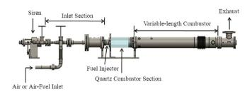
Fig. 7. Schematic diagram of the combustor apparatus.
