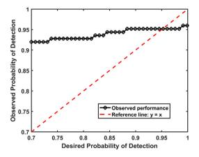
**Fig. 11.** Observed probability of detection for different values of desired probability of detection  $(p_d)$  and constant probability of false alarm  $(p_{fa}) = 0.01$  using experiment data.
