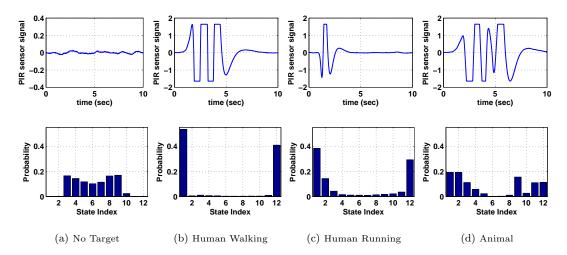
**FIGURE 1.16**: Examples of PIR sensor measurements (top) and the corresponding feature vectors extracted by SDF (bottom) of the four classes
