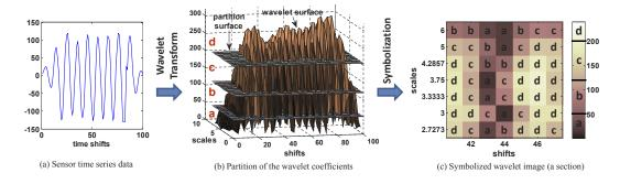
**FIGURE 1.1**: Symbol image generation via wavelet transform of the sensor time series data and partition of the wavelet surface in ordinate direction
