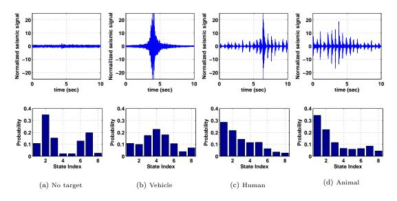
**FIGURE 1.14**: Examples of seismic sensor measurements (top) and the corresponding feature vectors extracted by SDF of the four classes (bottom)
