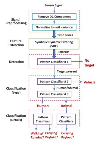
FIGURE 1.13: Flow chart of the problem of target detection and classification
