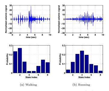
**FIGURE 1.15**: Examples of seismic sensor measurements (top) and the corresponding feature vectors extracted by SDF (bottom) for human walking and running
