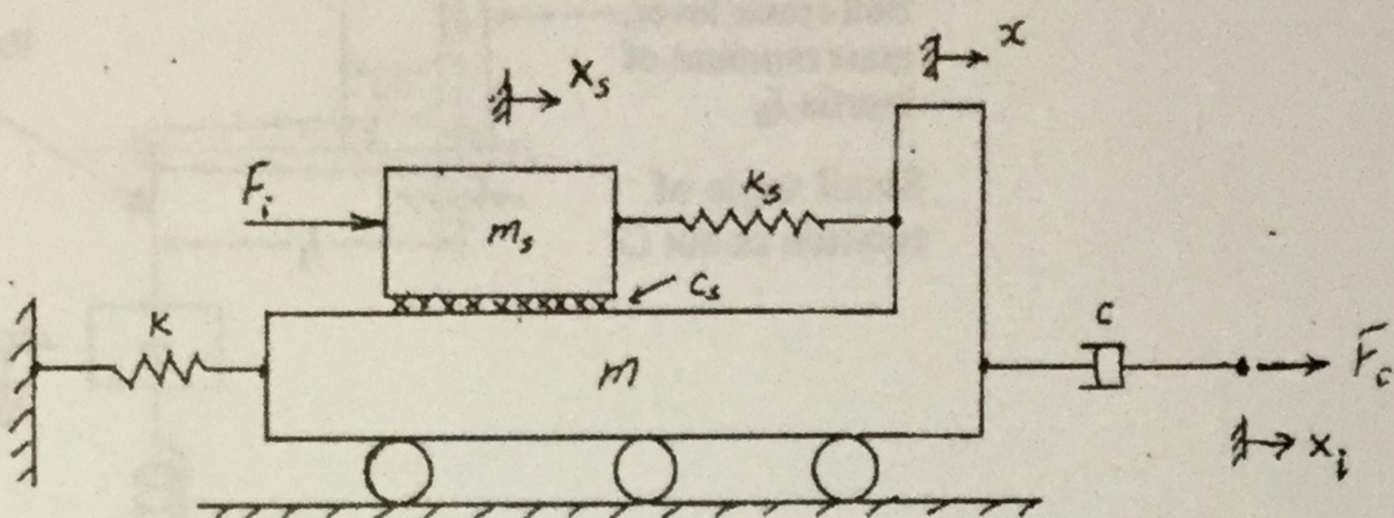
Draw the FBDs of all the model elements given below with **force and motion variables**. Make sure all FBDs are **complete** and **consistent** with the forces,  $F_{cs}$ ,  $F_{ks}$  and  $F_k$ , labelled on the incomplete FBDs of the two masses. Pay attention to action/reaction pair of forces between two connected elements.
