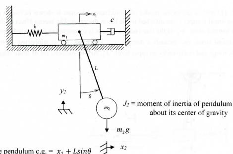
$x_2$  = x-position of the pendulum c.g. =  $x_1 + L\sin\theta$  $y_2$  = y-position of the pendulum c.g. =  $L - L\cos\theta$
