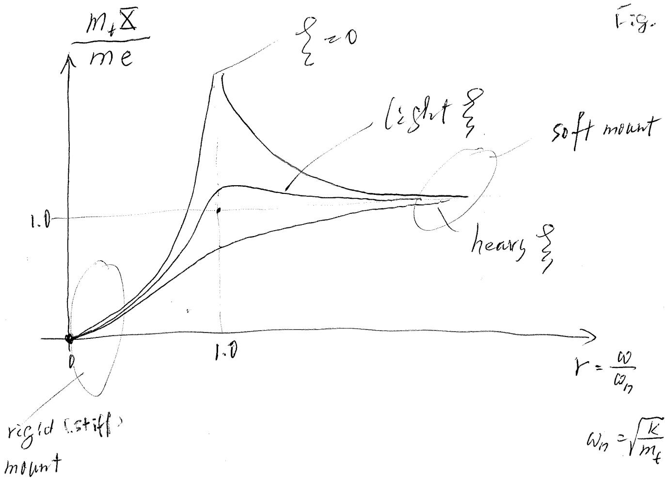
b) Magnitude of force transmitted to machine foundation:
