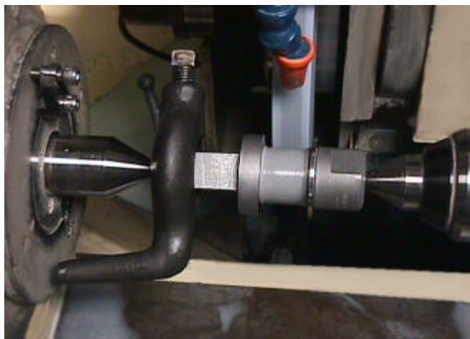
Figure 6. Preparing to grind the wear specimen, mounted between centers, on the Weldon grinder.
