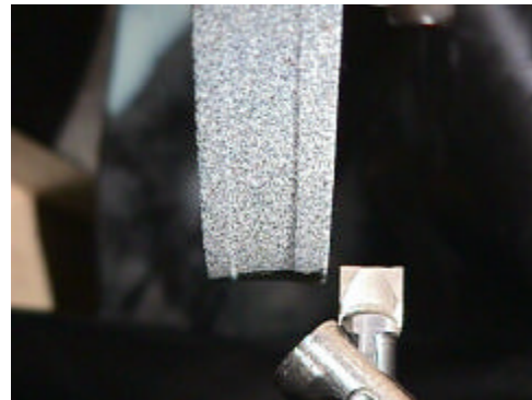
Figure 3. Grinding wheel and Multi-cut truing/dressing tool prior to truing the wheel.
