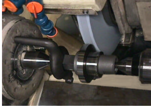
Figure 4. The Weldon grinder shown with 52100 steel test part mounted between centers.
