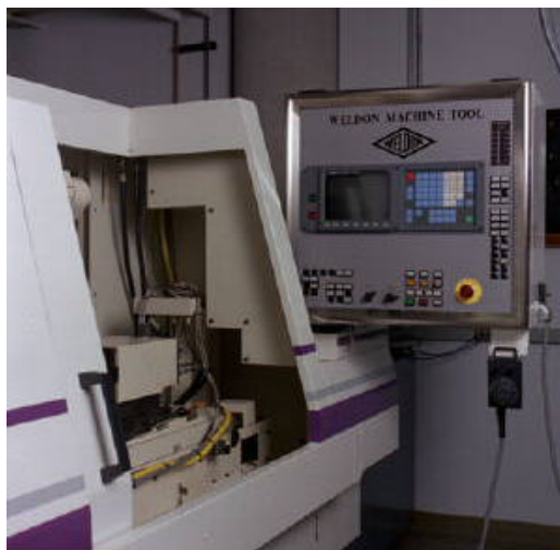
Figure 1. The Weldon Model AGN5 CNC cylindrical grinder.
