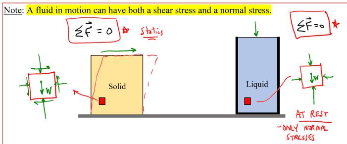
Examine all the stresses on a little element of the solid or the liquid by using a **free-body diagram**.
