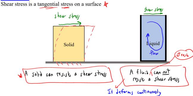
Bottom line: A fluid at rest cannot resist a shear stress.
