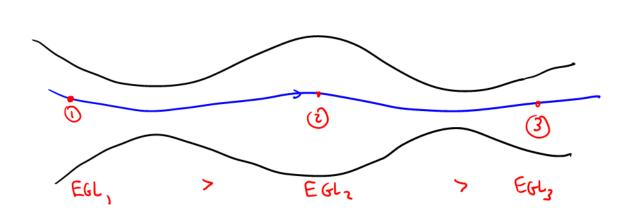
**Example: HGL and EGL (continued from above) Given:** Water at 20°C flows through a pipe. Two peizometers and two stagnation presssure probes are inserted into the pipe as sketched, and their column heights are measured from an arbitrary datum plane:
