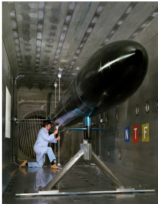
Submarine Tested in a Wind Tunnel. Image from NASA Langley.
