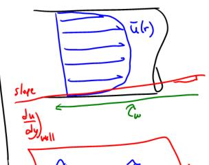
TURBULENT PIPE FLOW HAS A LANGER PRESSURE DROP FOR THE SAME FLOW RATE
