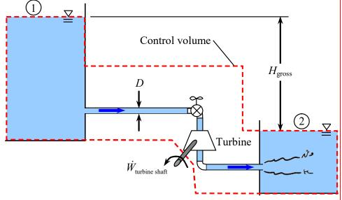
**To do**: Calculate the shaft power produced by the turbine in units of kilowatts.
