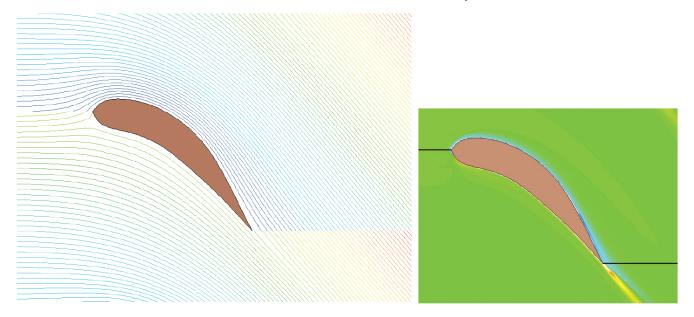
**Steady Three-Dimensional Flow**: This is flow through the stator blades of an axial flow fan (rotor blaces are downstream, not shown). Plotted are pressure contours.
