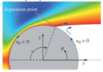
**Unsteady Two-Dimensional Flow**: This is laminar flow over a circular cylinder. Image (a) shows vorticity contours from CFD. Image (b) shows dye streaklines from experiment.
