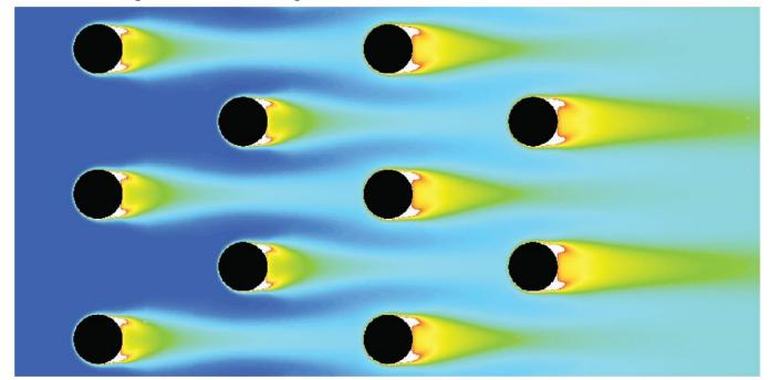
**Steady Three-Dimensional Flow with Heat Transfer**: This is flow over a printed circuit board, comparing chip surface temperature as a function of chip orientation. Shown below are the two configurations. Shown on the next page are boundary conditions and temperature contours.
