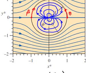
of  $\psi$ , i.e.,  $u_r = \frac{1}{r} \frac{\partial \psi}{\partial \theta}$   $u_\theta = -\frac{\partial \psi}{\partial r}$ . See text for details. On the cylinder (r = a),
