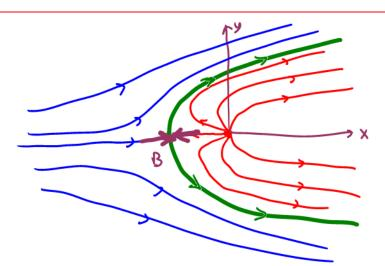
ANY STREAMLINE IN A POTENTIAL FLOW CAN BE THOUGHT OF AS A WALL
