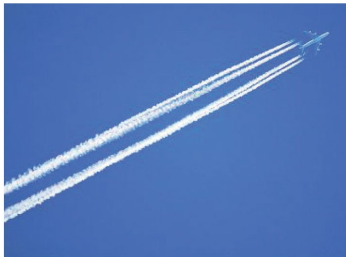
Four contrails merge into two trailing vortices.
