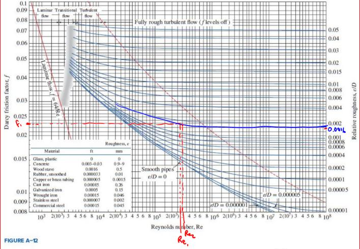
The Moody chart for the friction factor for fully developed flow in circular pipes for use in the head loss relation  $h_L = f \frac{L}{D} \frac{V^2}{2g}$ . Friction factors in the turbulent flow are evaluated from the Colebrook equation  $\frac{1}{\sqrt{f}} = -2 \log_{10} \left( \frac{e/D}{3.7} + \frac{2.51}{\text{Re } \sqrt{f}} \right)$ .
