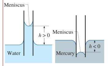
We can predict the rise height has a function of contact angle and surface tension, along with other parameters like inner tube diameter, liquid density, and gravitational constant:
