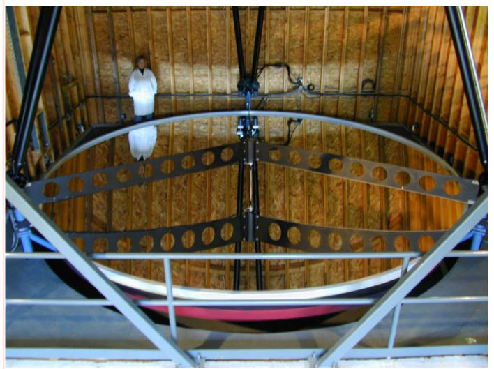
Mirrors made from spinning molten glass in a furnace, and letting it harden in the paraboloid shape.
