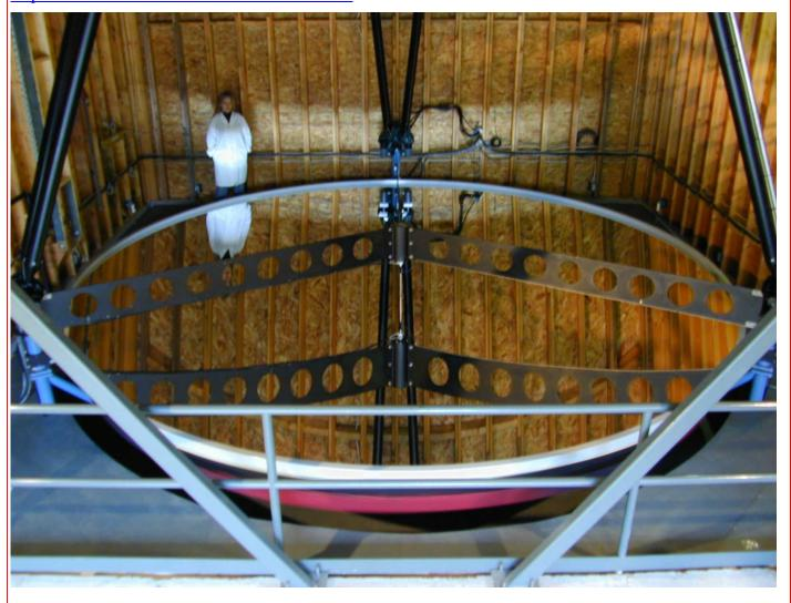
Mirrors made from spinning molten glass in a furnace, and letting it harden in the paraboloid shape.
