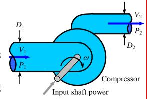
(a) **To do**: Calculate the average velocity of the air entering the compressor.
