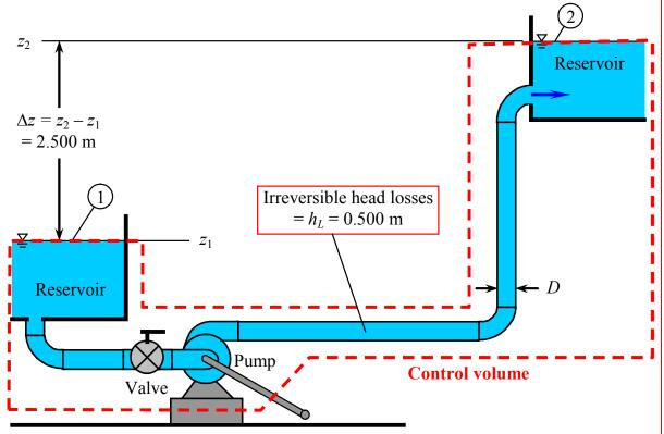
**To do**: Calculate  $h_{pump,u}$ , the useful pump head supplied to the water in meters of water.
