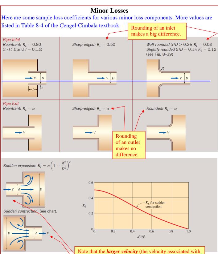
Note that the *larger velocity* (the velocity associated with the *smaller pipe section*) is used by convention in the equation for minor head loss,  $h_{L, \text{minor}} = K_L \frac{V^2}{2\sigma}$ .
