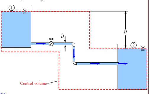
To do: Calculate the volume flow rate through this piping system.
