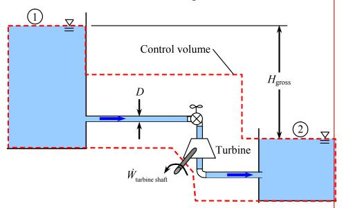
turbine is 81% efficient. The volume flow rate through the turbine is  $0.0045 \text{ m}^3/\text{s}$ .
