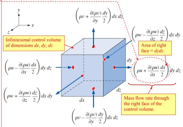
Next, we add up all the mass flow rates through all six faces of the control volume in order to generate the general (unsteady, incompressible) *continuity equation*:
