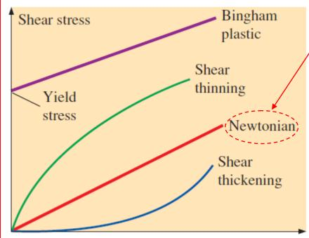
For **Newtonian fluids**, the shear stress is linearly proportional to the shear strain rate.
