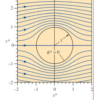
of  $\psi$ , i.e.,  $u_r = \frac{1}{r} \frac{\partial \psi}{\partial \theta}$   $u_\theta = -\frac{\partial \psi}{\partial r}$ . See text for details. On the cylinder (r = a),  $u_r = 0$   $u_\theta = -2V_\infty \sin \theta$
