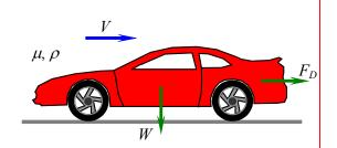
**To do**: Estimate the power requirement of the engine (in kW) delivered to the wheels.
