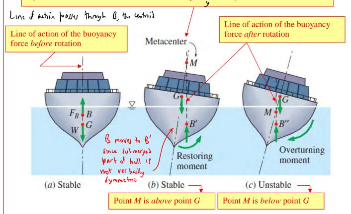
Bottom line: The boat is unstable if metacenter M is below center of gravity G.
