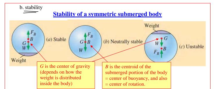
Bottom line: The body is unstable if center of buoyancy B is below center of gravity G.
