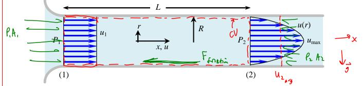
**To do**: Calculate the total friction force acting on the fluid by the pipe wall from 1 to 2. **Solution**:
