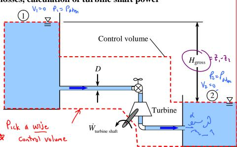
turbine is 81% efficient. The volume flow rate through the turbine is 0.0045 m<sup>3</sup>/s.
