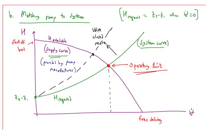
The flow will automatically adjust styll to this operating point
