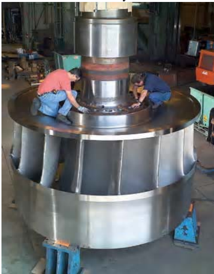
Francis mixed-flow hydroturbine:
