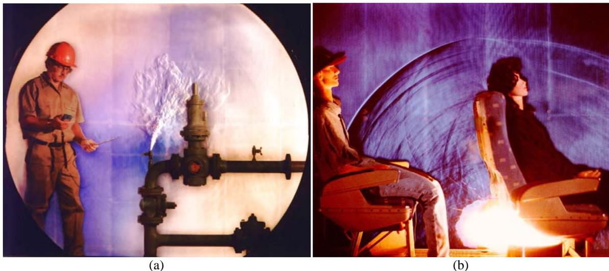
**Figure 6.** Color schlieren images from the full-scale system at the PSGDL: (a) propane gas leaking from a valve, modeled by J. D. Miller, and (b) explosion beneath a full size aircraft seat occupied by a dummy. This photo aided in the research (funded by the FAA) of aircraft hardening in response to incidents of international terrorism. Photos courtesy of G. S. Settles.
