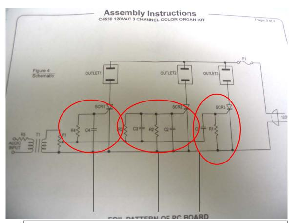
As shown in the lecture slides, these are good examples of a low-pass, band-pass, and high pass filter from left to right. Note: the band-pass combines both low and high – showing 2 capacitors.
