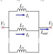
their magnetic fields interact with each other, there is an additional effect called *mutual inductance*. If the mutual inductance is significant, the above equations for series and parallel inductors are no longer reliable.
