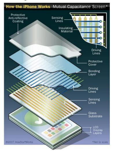
A mutual capacitance touch-screen contains a grid of sensing lines and driving lines to determine where the user is touching.
