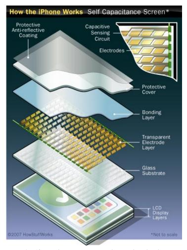
A self capacitance screen contains sensing circuits and electrodes to determine where a user is touching.
