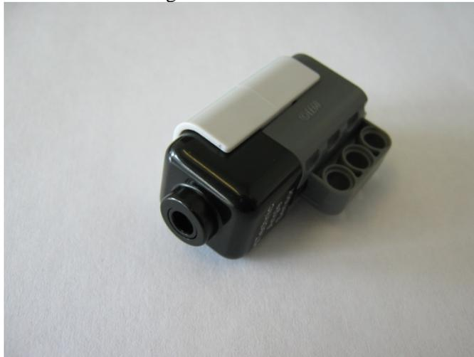
**Figure 1: Lego angle sensor**
