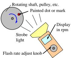
stroboscopic tachometer, except electronics remove the manual component.
