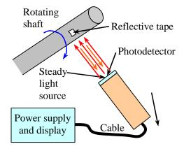
**Photoelectric tachometer:** This instrument is somewhat similar in principle to the
