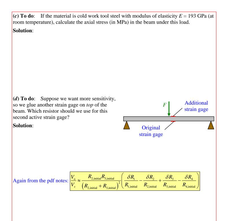
(e) To do: For the setup of Part (d) with the same strain as in Part (b), calculate output voltage  $V_0$ .
