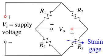
(a) To do: Will  $V_0$  be positive or negative when a downward load is added? Solution:
