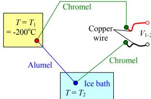
**To do**: Calculate the temperature that Fred measures, and the percentage error. Use the "brief" thermocouple tables for consistency.
