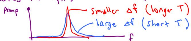
(2) Windowing → Consider the middle portion of the signal as more important than the beginning & end of the signal
