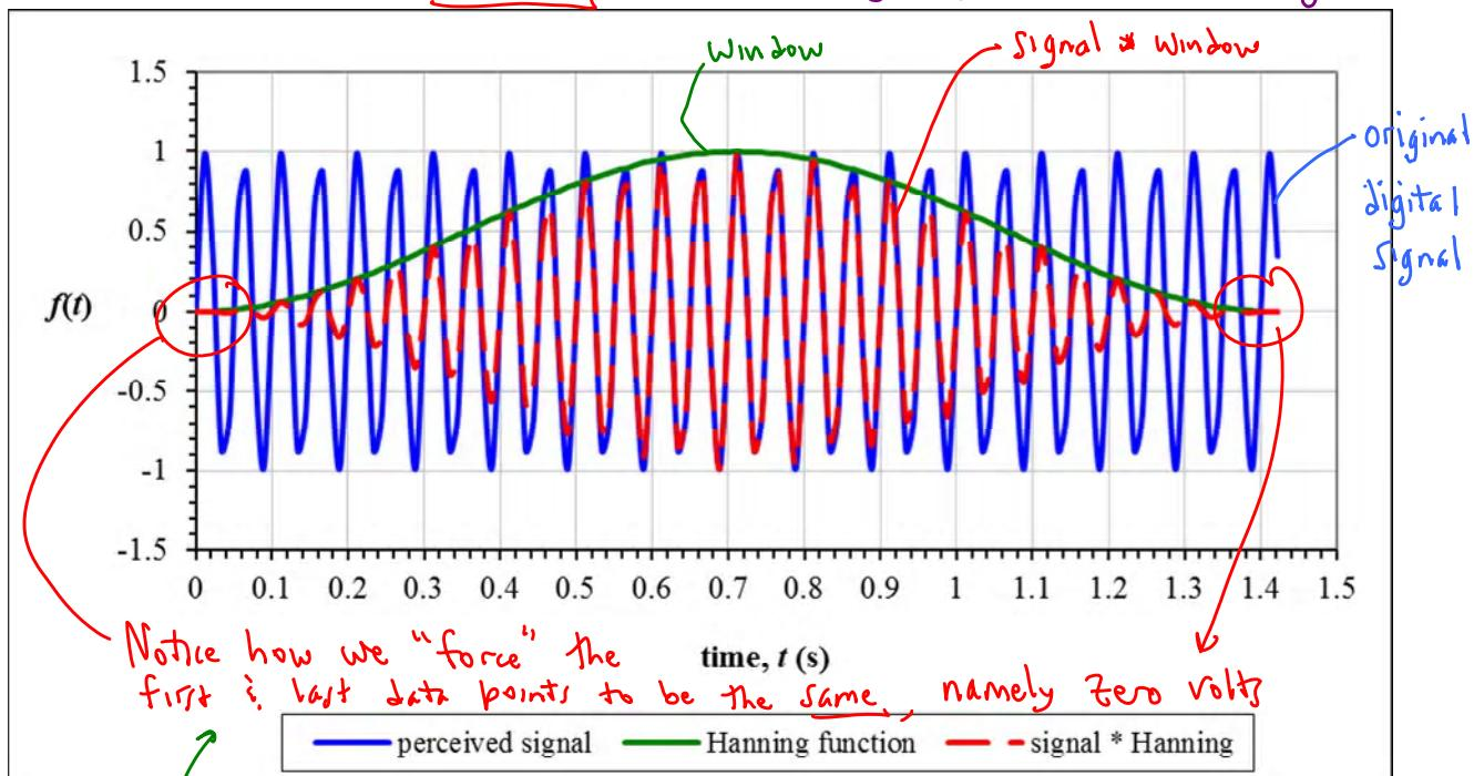
Windowing reduces leakage since now the first & last data pts are the same (zero volts)
