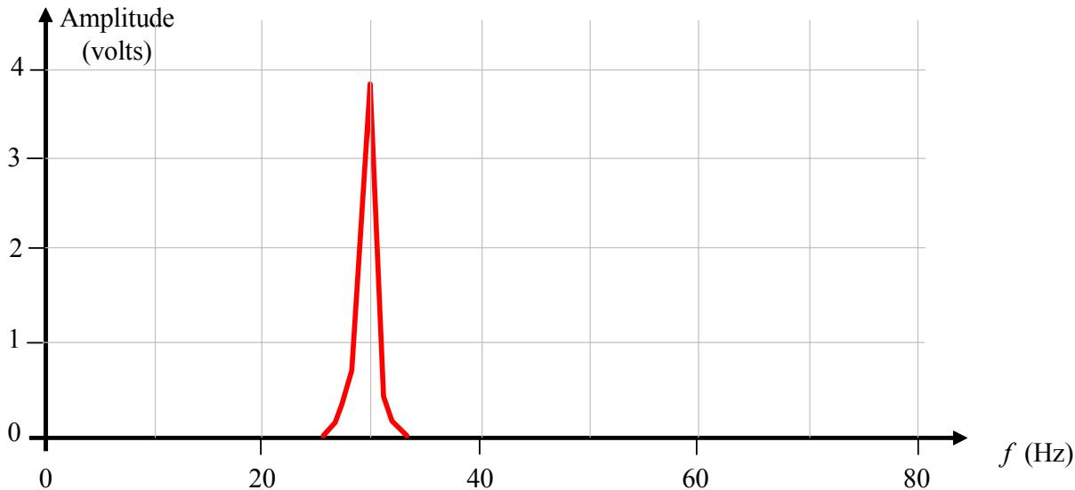
We conclude that there is a frequency component of about 30 Hz, with an amplitude of about 4 volts. But how can we be sure? What if the 30 Hz peak is *aliased* from some higher frequency?
